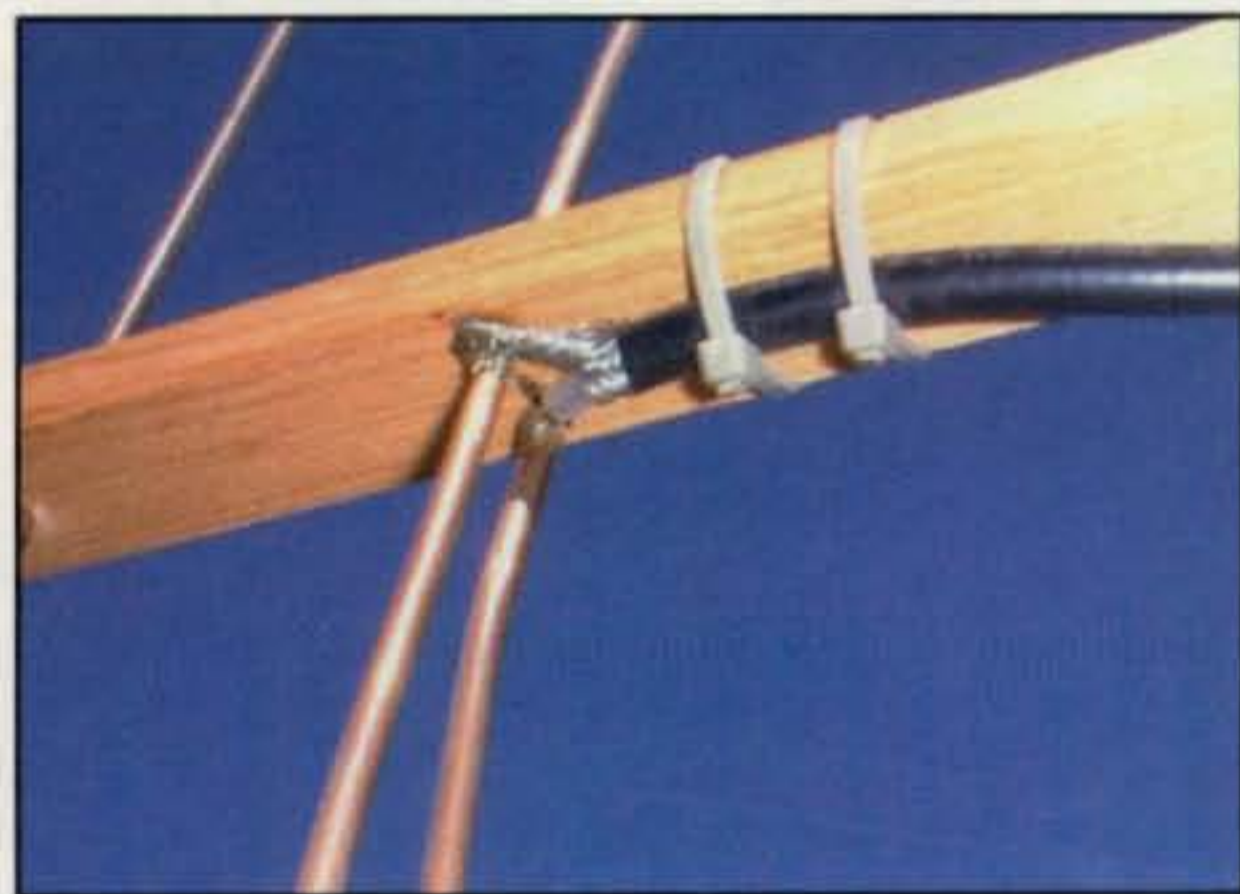
Photo A— Driven element and coax.
