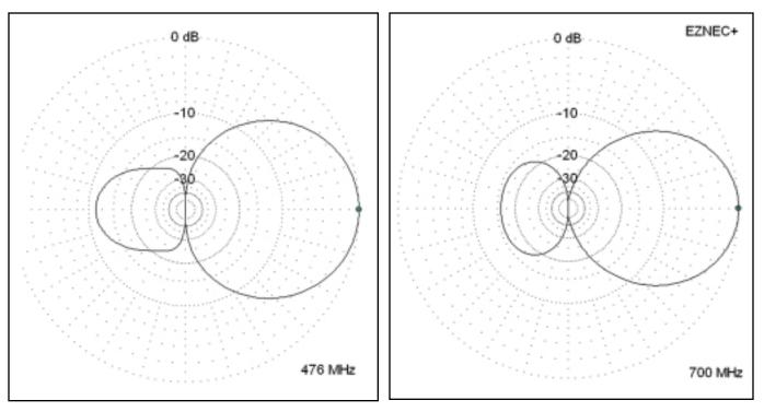
Figure 1. EZ HDTV pattern on UHF TV Channel 14.
