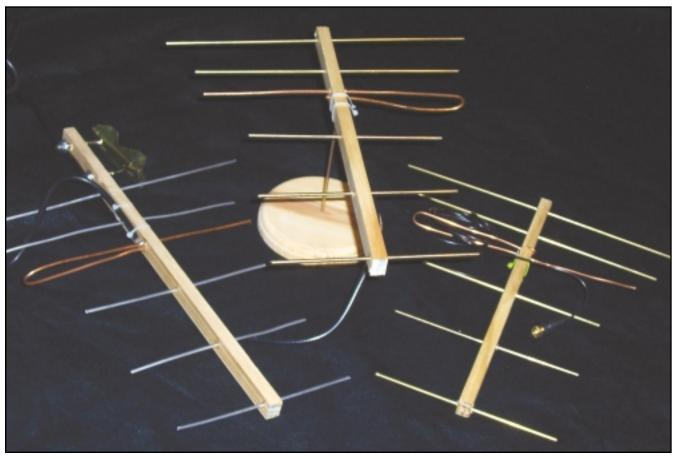
Photo A. Easy-to-build HDTV antennas.
