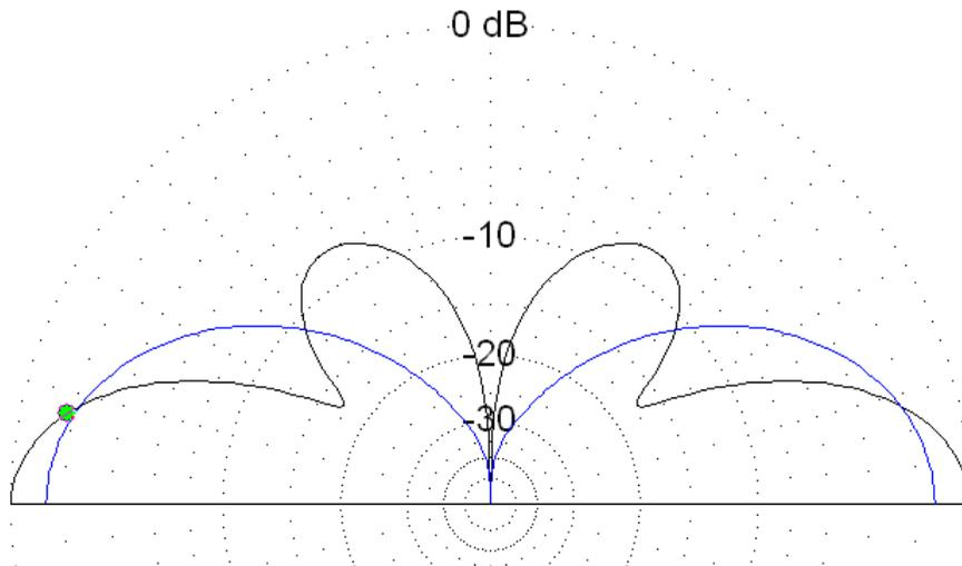
But if you bend up a 3/4ths length of wire until it is 5/8ths wave long, we get a very nice pattern back at the horizon as also shown above. The loop, or partial loop in the center element is not a loading coil like you might see on many HF antennas. In this case it is a delay line. It is instead a way of delaying the wave so that it is seeing  $\frac{3}{4}$  ths wavelength in a  $\frac{5}{8}$  wavelength space. This delay line can be a loop, part of a loop, a stub, or a zig-zag.
