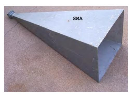
wave on that frequency. For 700 MHz that works out to when the throat of the horn just over 200 mm wide.
