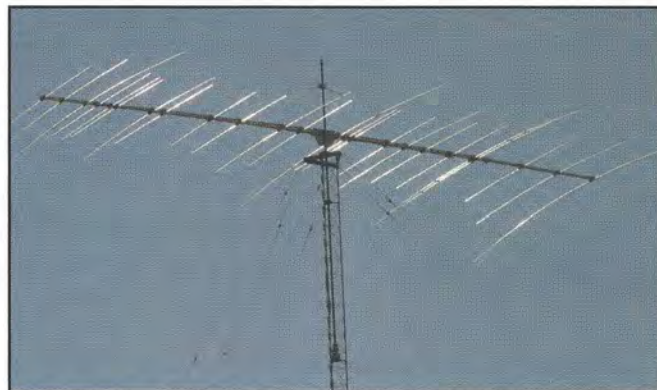
Photo F— This Force 12 multiband HF Yagi has elements for different bands so close they're on the same boom! (Courtesy of Force 12 Antennas)
