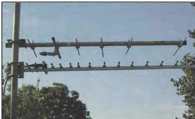
Photo D— Measuring a 915-MHz Yagi and its interaction with a 440-MHz Yagi.
