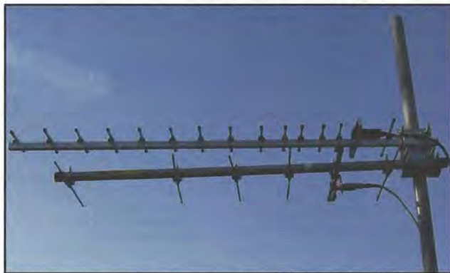
Photo B— Spacing before we saw \frac{1}{4} -dB drop in forward gain.
