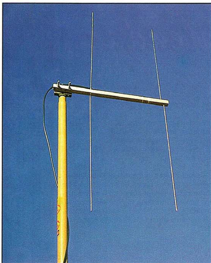
Photo A. The two-element air band Yagi.
