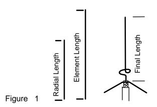
Using Figure 1, cut your center element to length. Now bend it around a small screwdriver, drill bit, etc until the total length is correct per chart 1. Now solder the element to the center of the coax.
