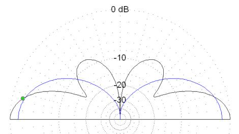
But if you bend up a 3/4ths length of wire until it is 5/8ths wave long, we get a very nice pattern back at the horizon as also shown above. The loop, or partial loop in the center element is not a loading coil like you might see on many HF antennas. In this case it is a delay line. It is instead a way of delaying the wave so that it is seeing <sup>3</sup>/<sub>4</sub> ths wavelength in a 5/8 wavelength space. This delay line can be a loop, part of a loop, a stub, or a zig-zag.
