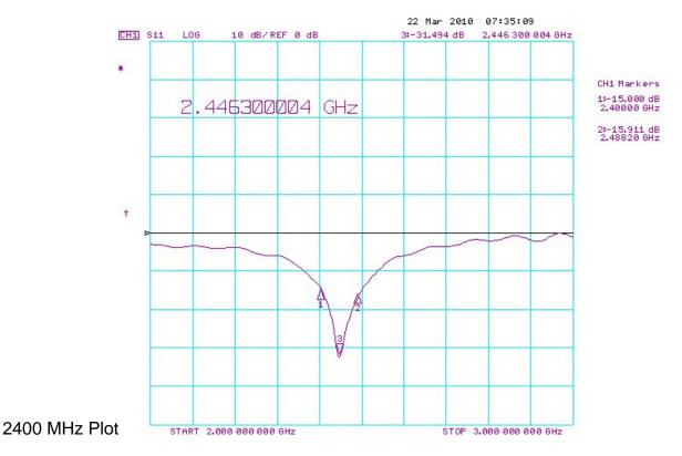
Here is the Network analyzer plot of the 2.4 GHz antenna.
