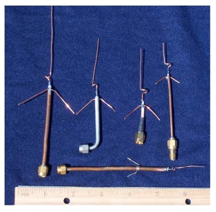
Here are some easy to build 5/8ths antennas for the 2.4 GHz, 3.4 GHz, and 5.8 GHz bands. These can be used with WiFi, 802.11, Zigbee, ATV, Bluetooth, and any other services on these bands.
